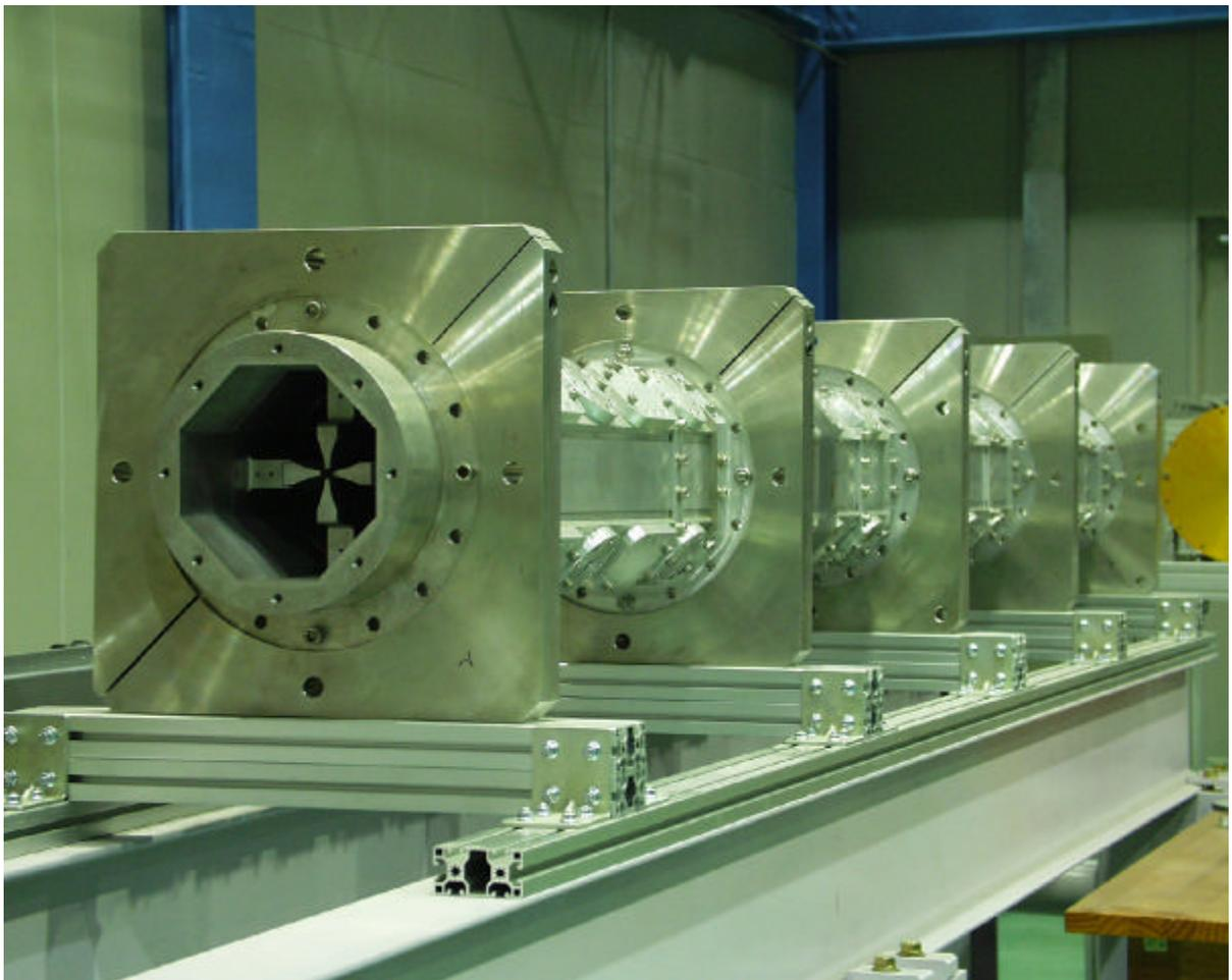
Figure 1. 3.0MeV KTF/RFQ consists of two resonantly coupled segments.
