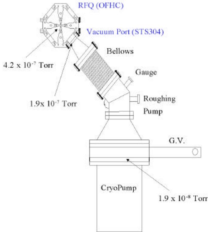
Figure 2. Schematic diagram of the pumping stations and roughing system for section of RFQ.
