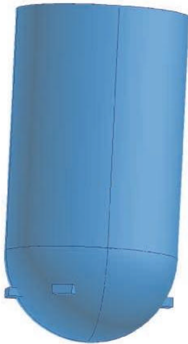
Figure 1 Schematic diagram of the shear keys attached to reactor vessel
