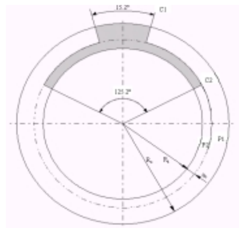
Fig. 10 Cracked pipe split by two co-centered pipes P1 and P2
