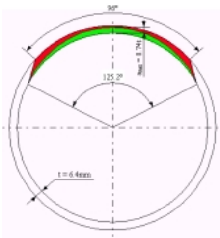
Fig. 9 Crack shape before and after the wall penetration
