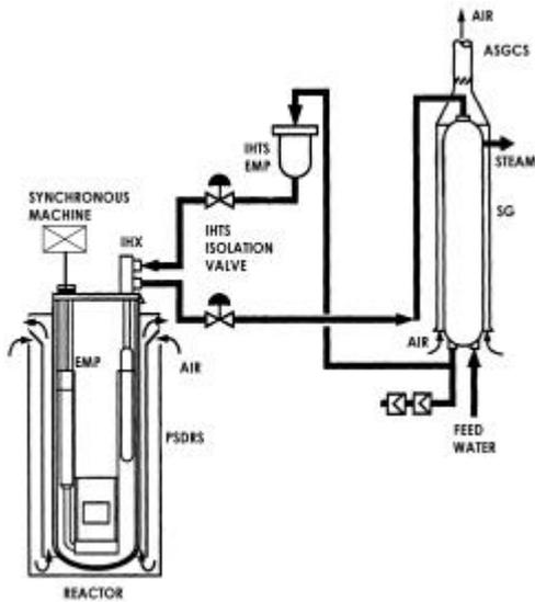
Fig. 3 Schematic Diagram of the PSDRS
