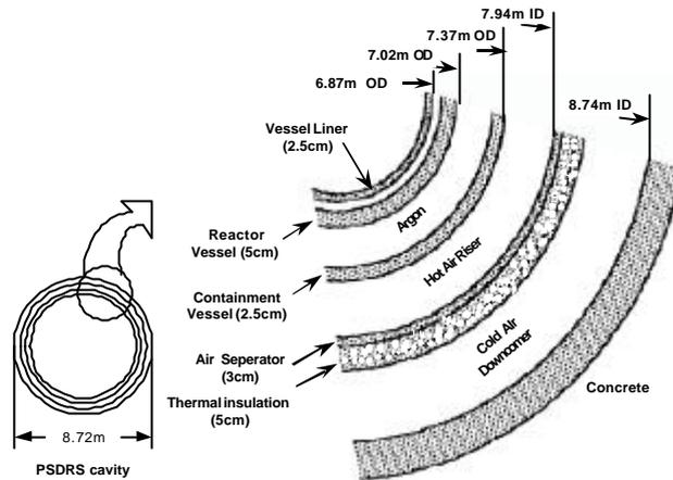
Fig. 4 Cross-sectional Flow Areas of the PSDRS
