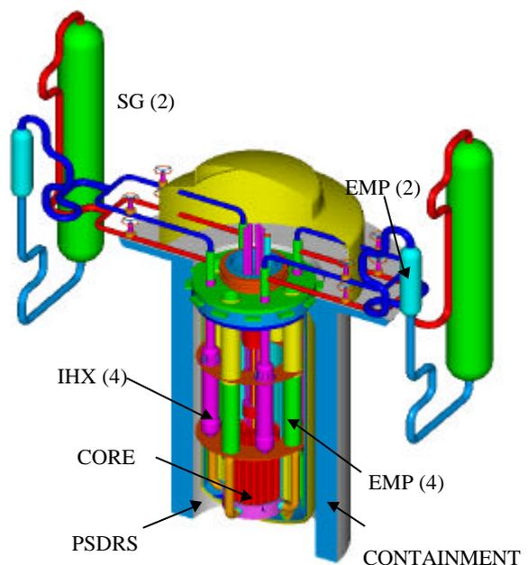
Fig.1 Schematic of the KALIMER Reactor Vessel
