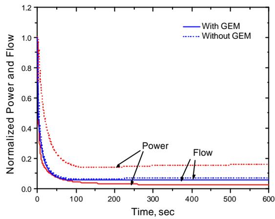
Fig.5 Power and flow fraction (ULOF)
