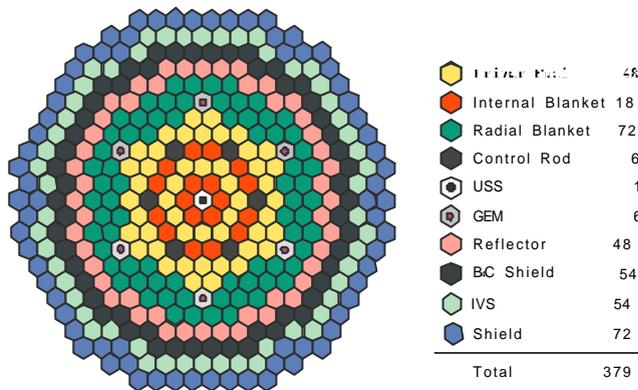
Fig.2 KALIMER Breeder Core
