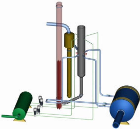
Fig. 1 Steam-Water DVI Test Facility
