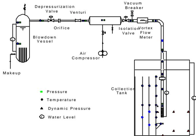
Fig. 4 Schematic Diagram of Unit Cell Sparger Test Facility
