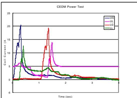
Fig. 6 CEDM Coil Current Trace
