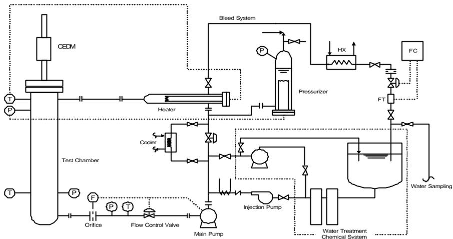
Fig. 5 KAERI CEDM Test Facility
