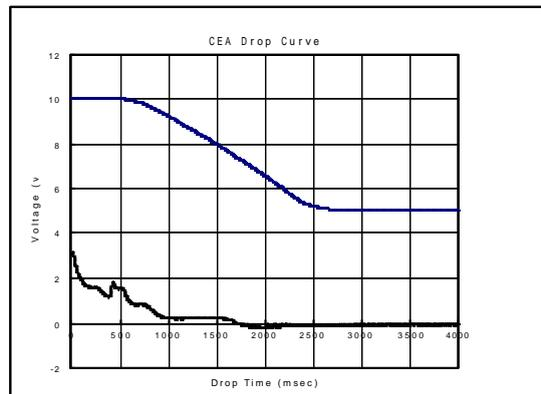
Fig. 7 Drop Curve of the Test Weight
