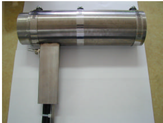
Figure 4. Dry ice snow jet cleaning machine
