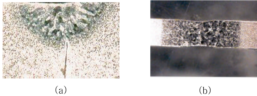
Fig. 11 Effect of defocusing on the weld formation
