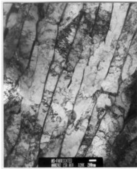
Fig. 1. Initial Microstructure of a Zr-2.5Nb tube operating in the Wolsong Unit 1 (Before Irradiation).
