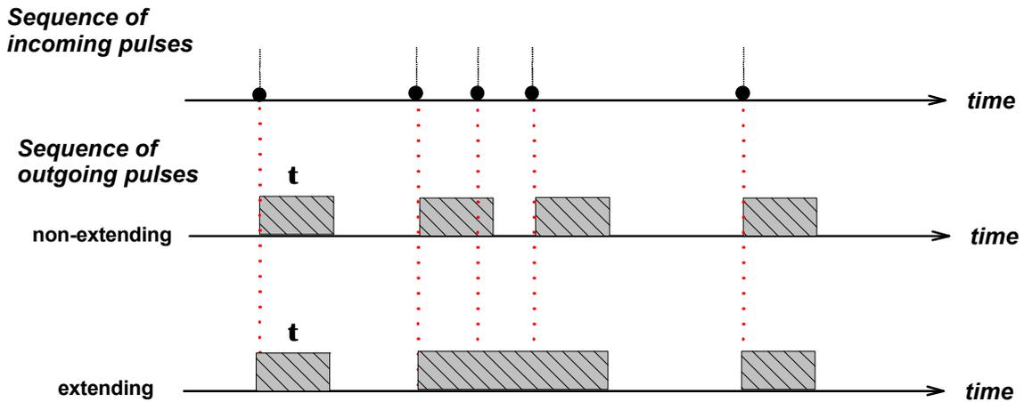
**Fig. 3 Illustrations of two types of Dead Times commonly applied in most experiments**
