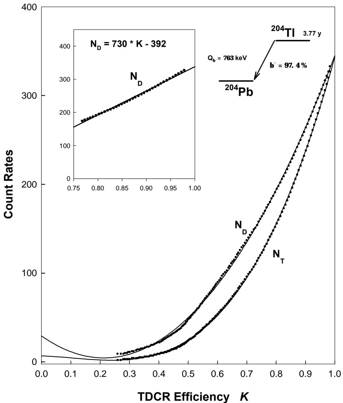
Fig. 7 Plots of  $N_D(K)$  and  $N_T(K)$  versus  $K$ . The data points were extrapolated to  $K = 1$  by the linear least-squares fit in the region of  $K \approx 75\%$ .
