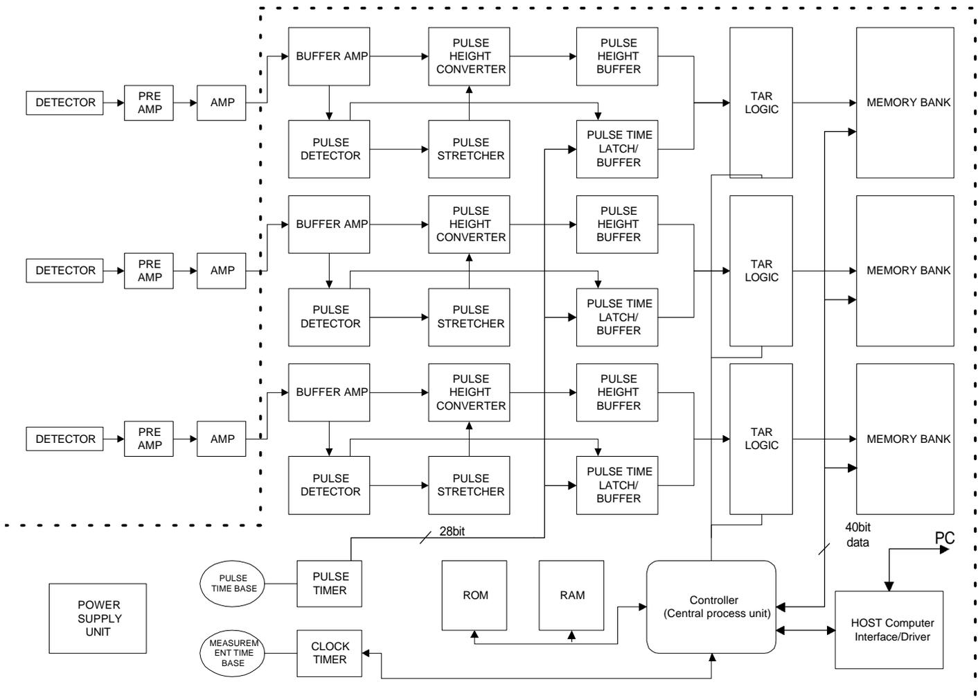
Fig. 2 Simplified block-diagrams of 3D-DAQ system
