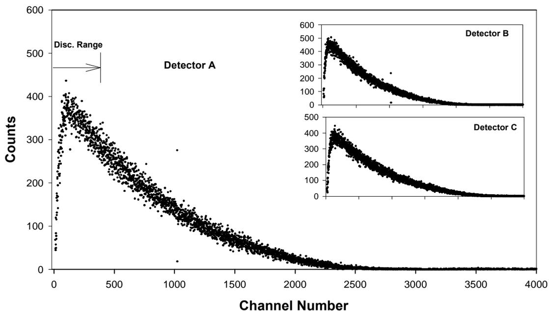
**Fig.5 Singles liquid scintillation spectrum of  $^{204}\text{Tl}$  obtained by using the 3-PM LSC at the present work. The computer discrimination range is marked on there.**
