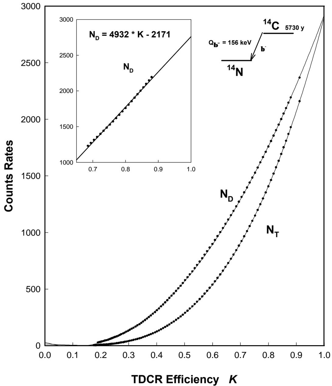
Fig. 6 Plots of  $N_D(K)$  and  $N_T(K)$  versus  $K$ . The data points were extrapolated to  $K = 1$  by the linear least-squares fit in the region of  $K \gtrsim 60\%$ .
