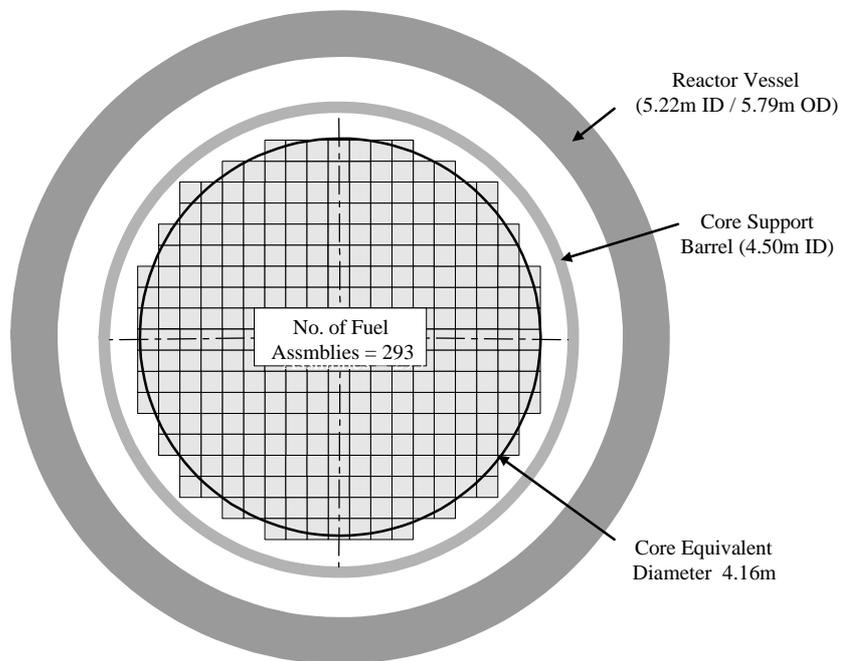
Figure 2. Cross-Sectional View of the Reactor (WH type)
