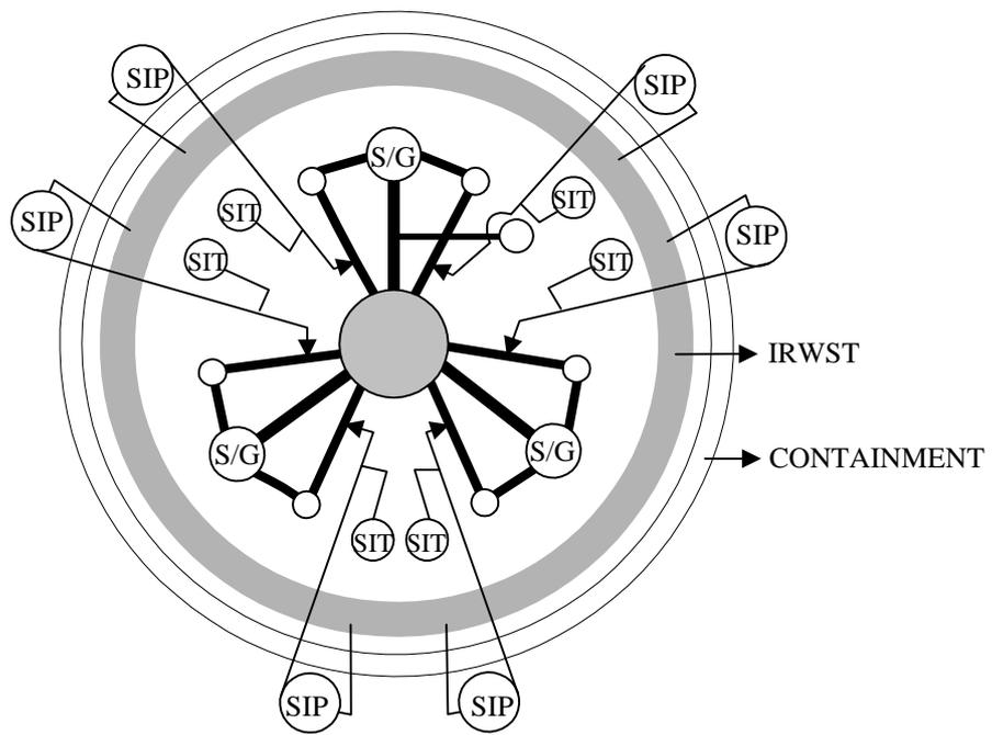
Figure 5. Arrangement of PWR-2000 RCS and CLI
