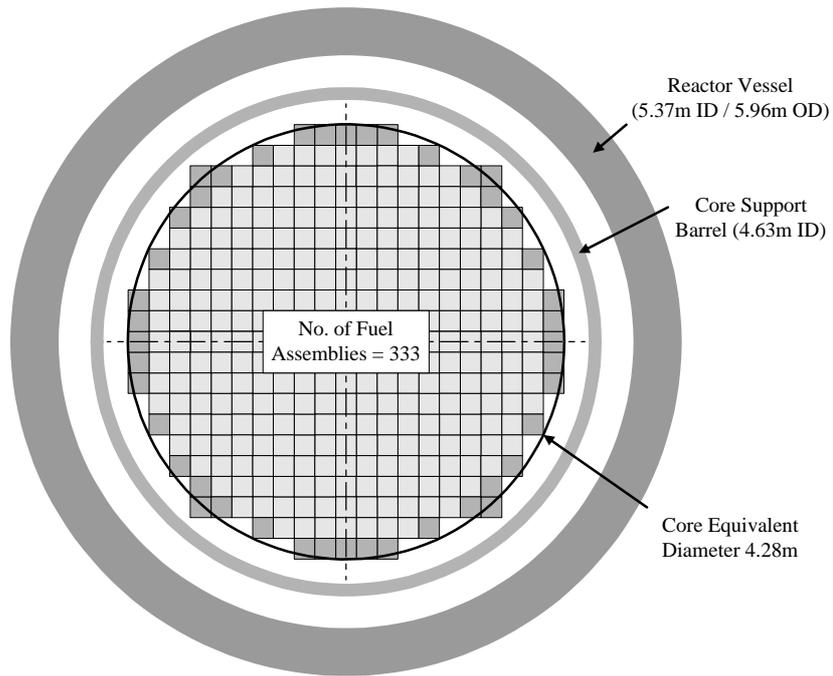
Figure 3. Cross-Sectional View of the Reactor (CE type)
