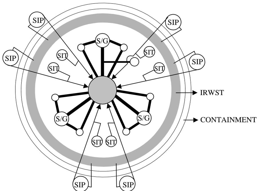
Figure 4. Arrangement of PWR-2000 RCS and DVI
