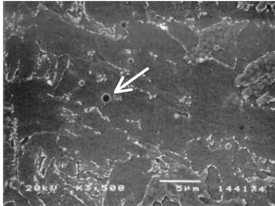
Fig. 3 SEM microstructure of the Linde 80 weld, K1W
