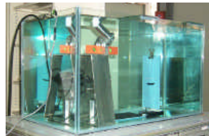
Fig. 7 Experimental set up for wall defect measurement
