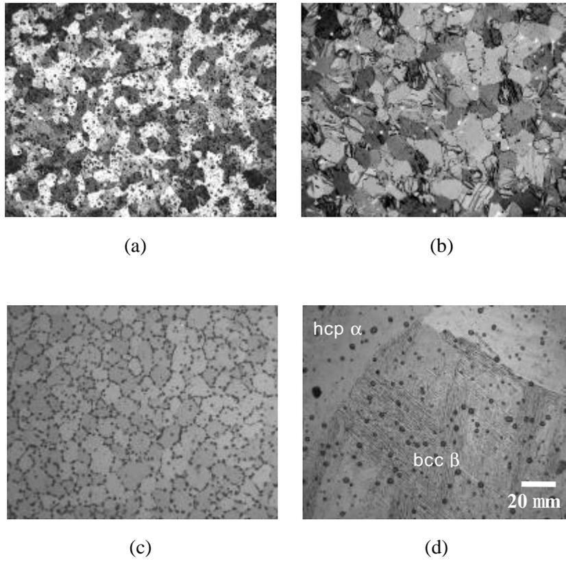
Fig. 1. Cross-sectional microstructures of as-received and heat treated PT-7M titanium alloy tubes: (a) as-received, and heat-treated at (b) 800, (c) 900, (d) 1000 for 1 hr.
