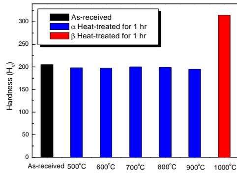
Fig. 7. Effect of heat-treatment on the hardness of PT-7M titanium alloy.
