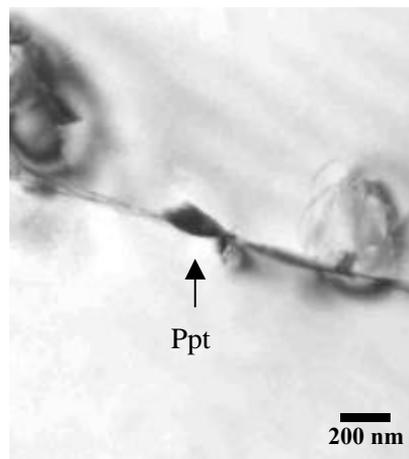
Fig. 4. Bright field TEM image of PT-7M titanium alloy heat-treated at 800 for 1 hr: Note that the precipitation size is much larger than that allowed in Fig. 3(a).
