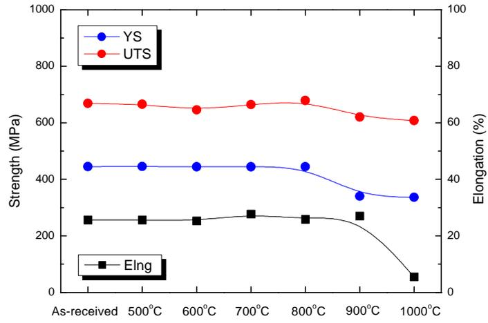
Fig. 5. Effect of heat-treatment on the tensile property of PT-7M titanium alloys.
