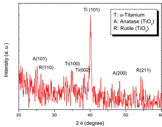
Fig. 9. X-ray diffraction pattern of PT-7M titanium alloy corroded at 360°C in the ammonia water chemistry of a pH 9.98 for 116 days.
