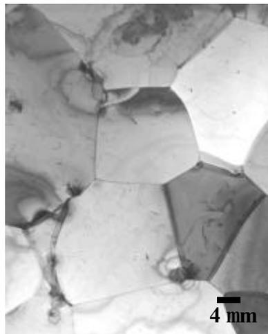
Fig. 2. Microstructure of the longitudinal section of as-received PT-7M titanium alloy tube.
