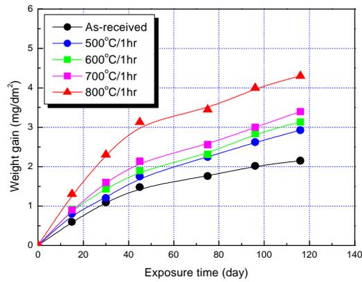
Fig. 8. Effect of  $\alpha$  heat-treatment on the corrosion behavior of PT-7M titanium alloy at 360°C in the ammonia aqueous solution of a pH 9.98.
