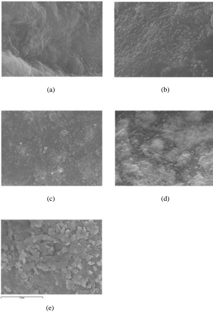
Fig. 10. SEM micrographs of oxide surfaces at the metal-oxide interfaces of PT-7M titanium alloys with equal weight gain of approximately  $2 \text{ mg/dm}^2$  grown in an ammonia aqueous solution of a pH 9.98: (a) as-received, and heat-treated at (b) 500 (c) 600 (d) 700 and (e) 800 for 1 hr.
