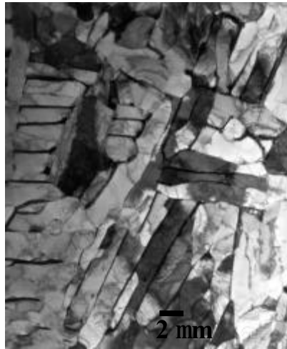
Fig. 3. Bright field TEM image of PT-3V titanium alloy ( \alpha+\beta Ti-alloy) showing a lamellar structure.
