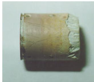
Fig. 4. Pellet of YSZ of 10mm Dia. X 10mm H.
