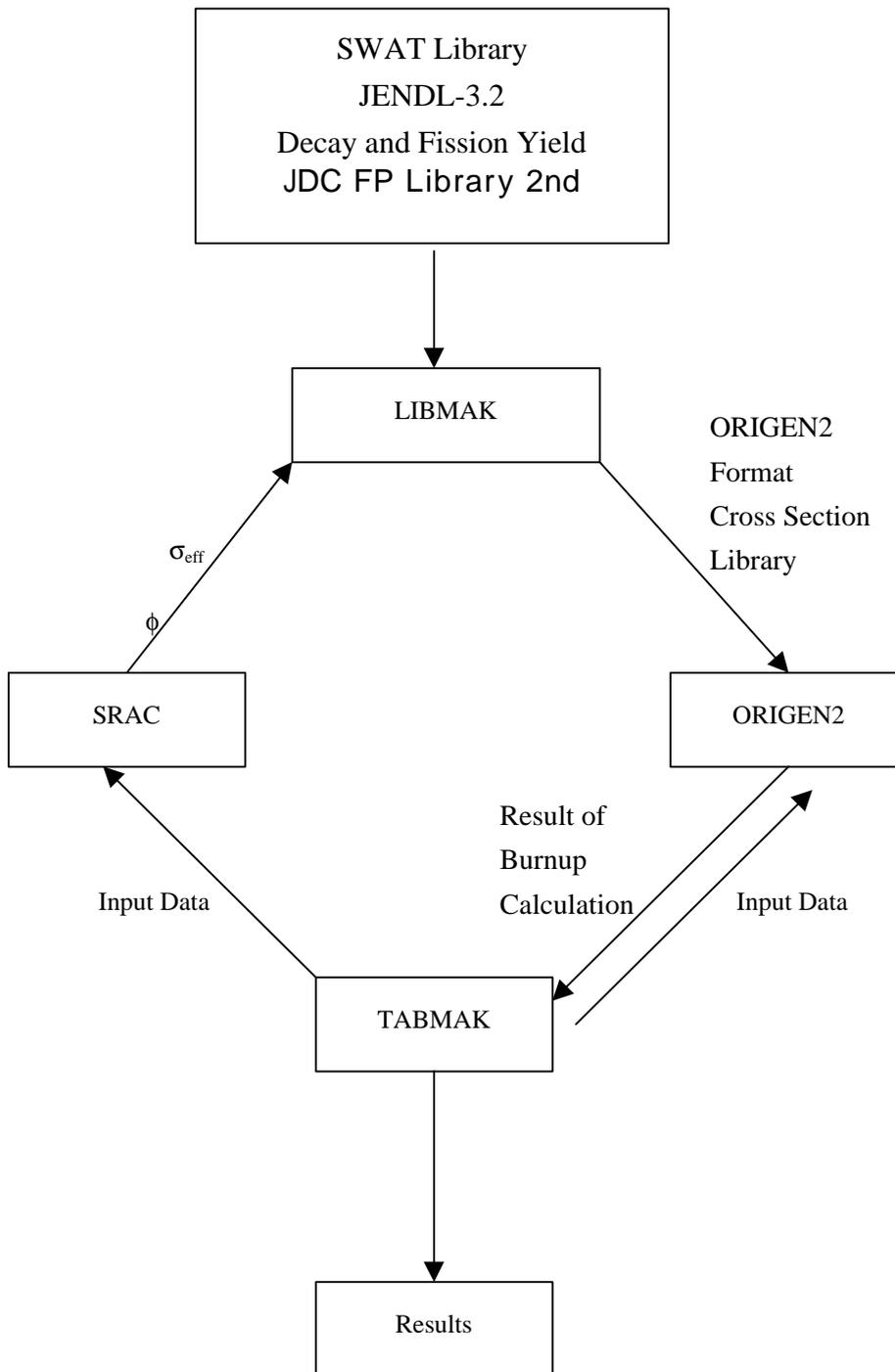
Fig. 1. Flow of Calculation in SWAT.
