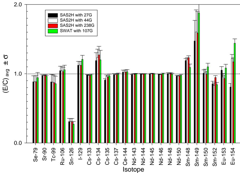
Fig. 9. Comparison of the Average Measured-to-Calculated Ratios and Standard Deviations for Fission Products.
