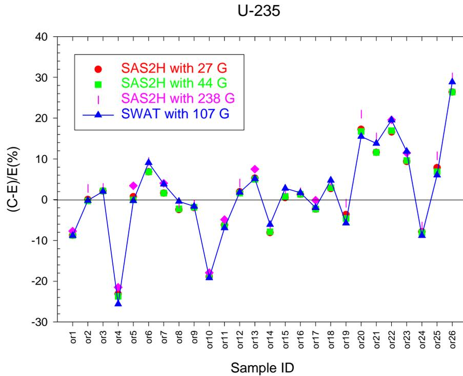
Fig. 3. Relative Errors of U-235 Calculated Compositions against Sample ID.
