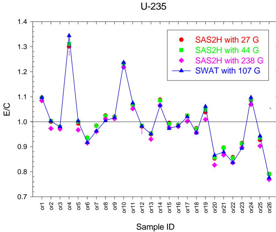
Fig. 2. Comparison of U-235 Measured-to-Calculated Ratios.
