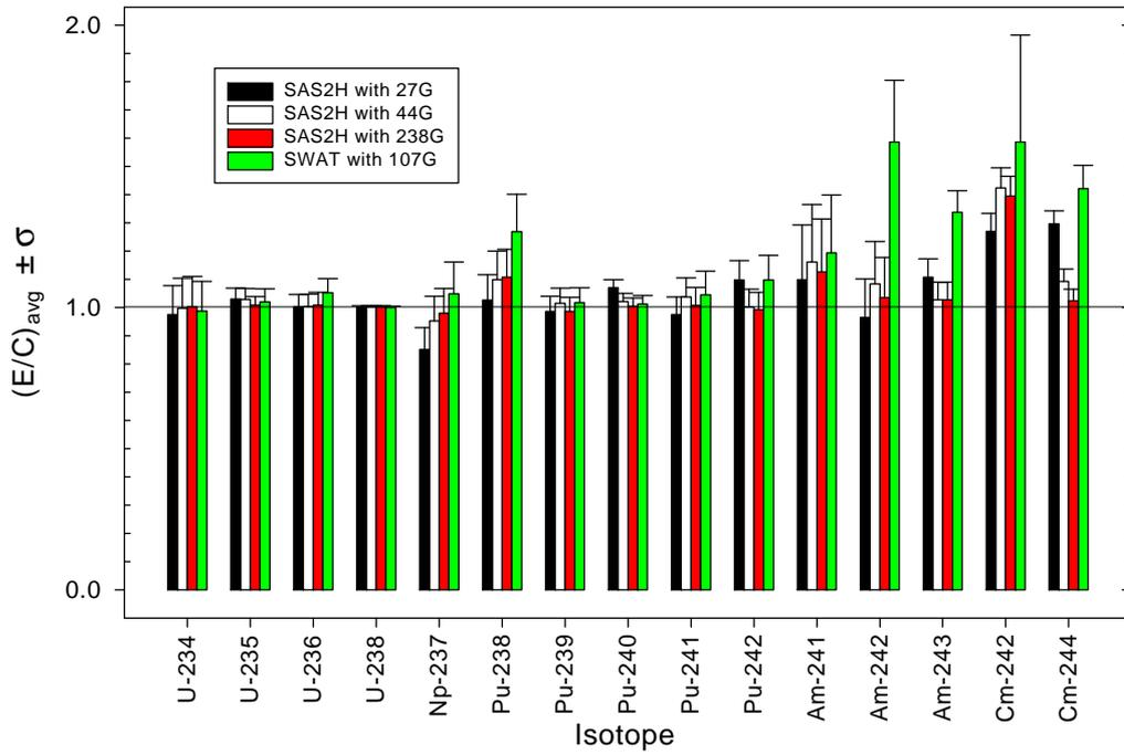
Fig. 8. Comparison of the Average Measured-to-Calculated Ratios and Standard Deviations for Actinides.
