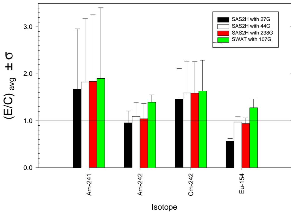
Fig.5. Comparison of the Average Measured-to-calculated Ratios and Standard Deviations for the large deviation nuclides.
