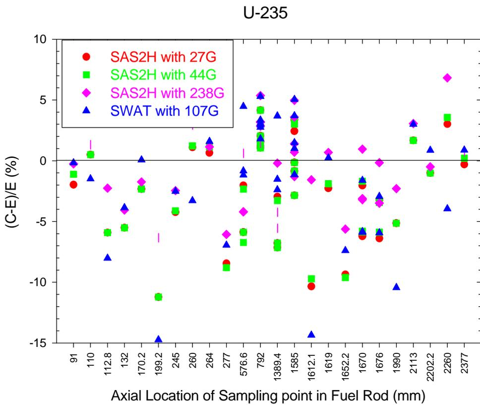
Fig. 7. Relative Errors of U-235 Calculated Compositions.
