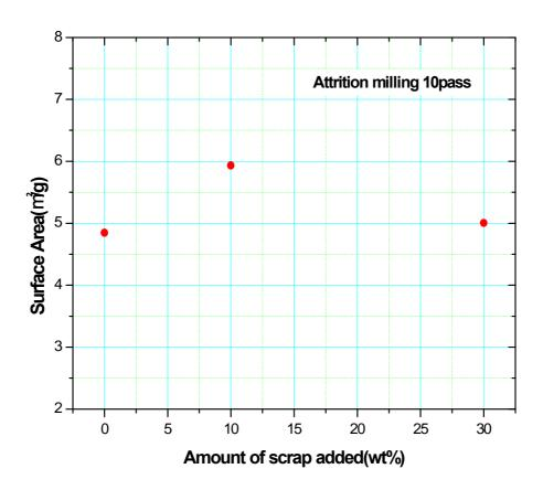
Fig. 3 Change of surface area of powder milled by attrition mill for each amount of  $MO_2$  scrap
