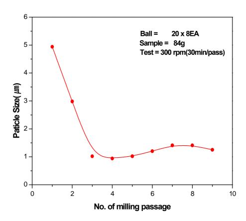
Fig. 1 Change of particle size of MO<sub>2</sub> scrap powder milled by planetary mill in each passage.
