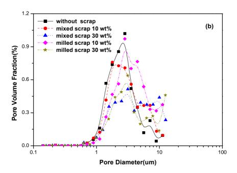
Fig. 6 Pore size distribution of  $(U, Ce)O_2$  pellets with the amount of  $MO_2$  scrap and doping methods:
