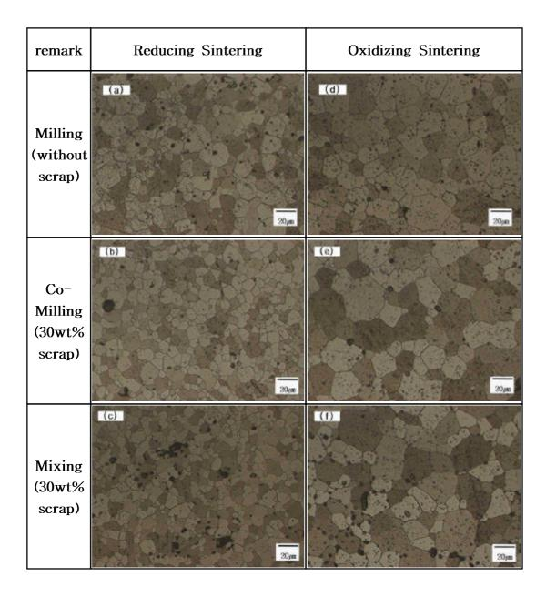
Fig. 5 Microstructure of (U, Ce)O<sub>2</sub> pellets in each condition:
