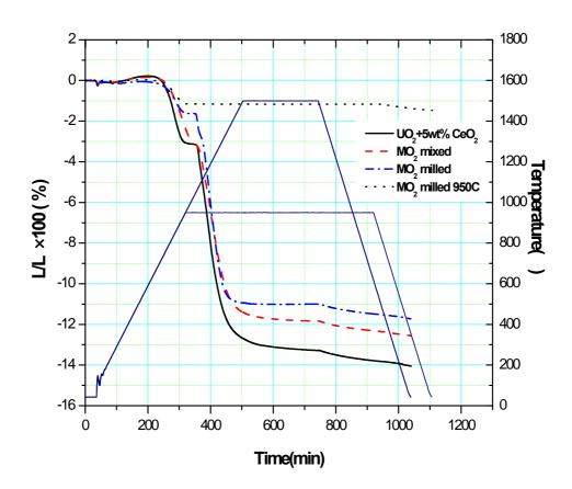
Fig. 7 TMA curves of MO<sub>2</sub> doped UO<sub>2</sub>+5wt%CeO<sub>2</sub>
