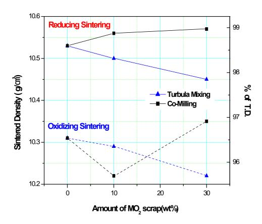
Fig. 4 Change in sintered density of (U, Ce)O<sub>2</sub> pellets with the amount of MO<sub>2</sub> scrap and different doping methods:
