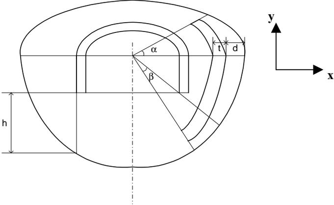
Fig. 7 Main design parameters of the target with a rectangular bypass.
