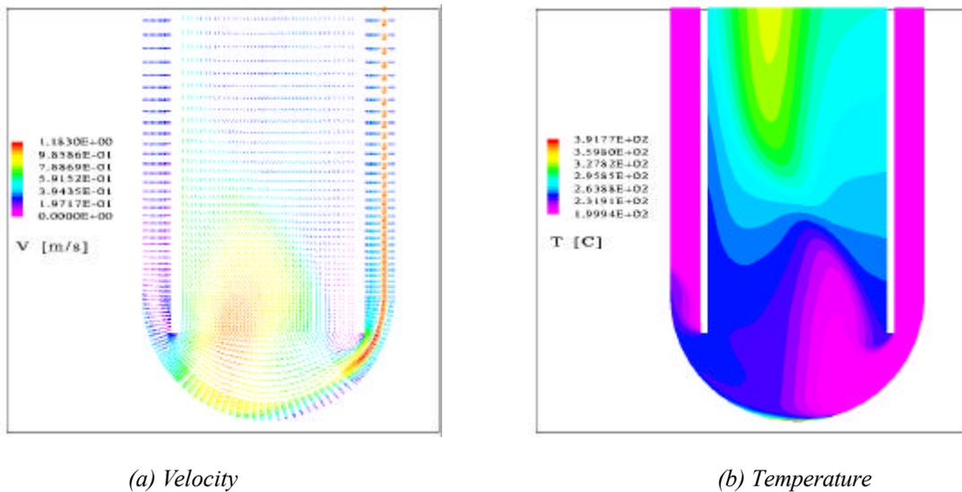
Fig. 8 Velocity and temperature distribution in the target with an injection bypass.
