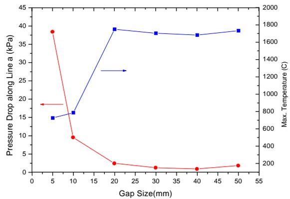
Fig. 5 Effects of the gap size on the pressure drop and the maximum window temperature.
