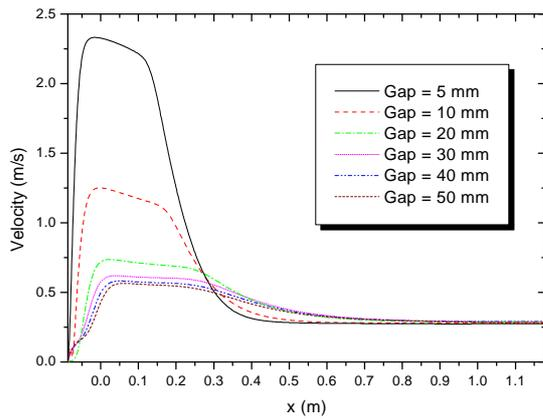
Fig. 4 Effects of the gap size on the velocity profile along the center line.
