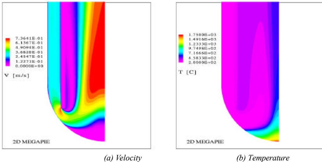
Fig. 3 Velocity and temperature distribution in the target with a flat guide tube and a gap size of 20 mm.
