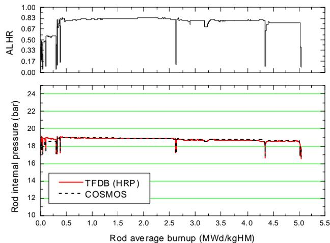
Figure 10. Comparison of COSMOS calculated RIP with measured values for MOX-ATT-TF
