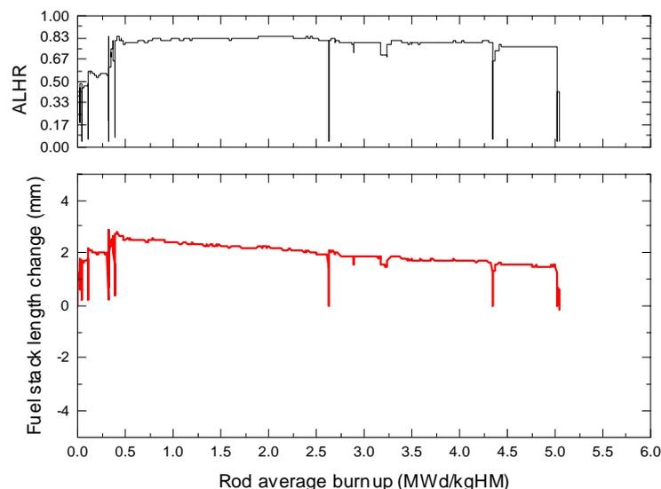
Figure 5. Measured stack elongation for MOX-ATT-TF.
