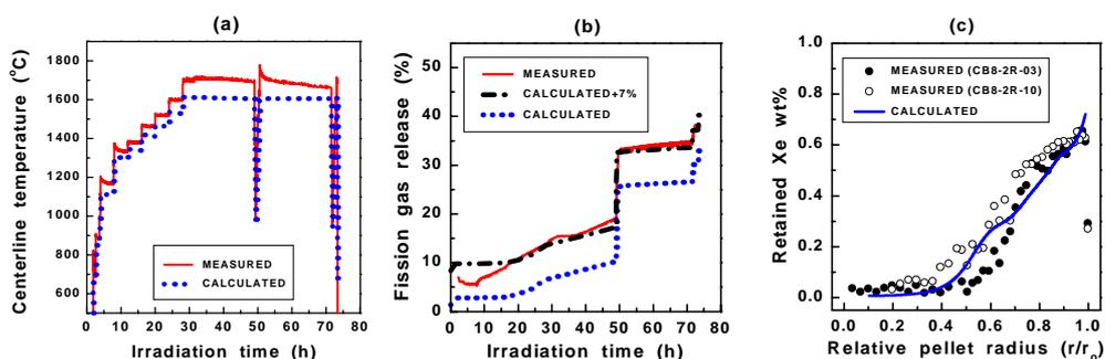
Figure 7. Analysis results for the Risø-III's AN3 test: (a) centerline temperature, (b) fission gas release and (c) radial distribution of Xe.
