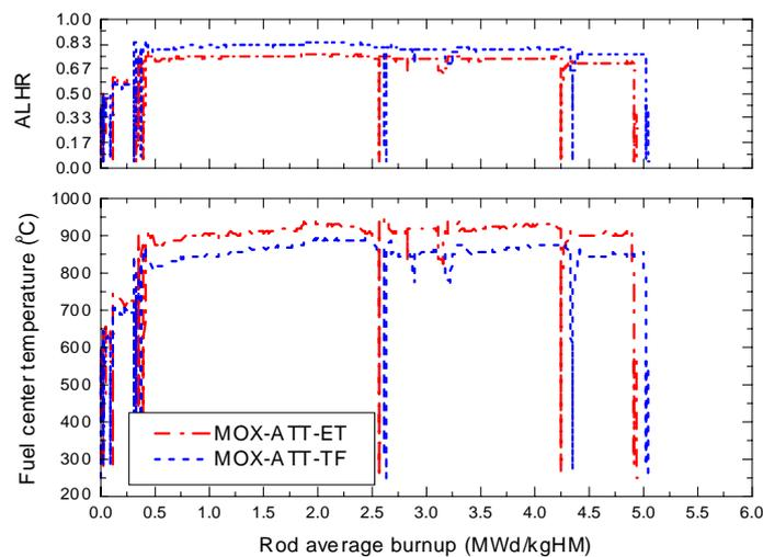
Figure 3. Measured fuel centerline temperature
