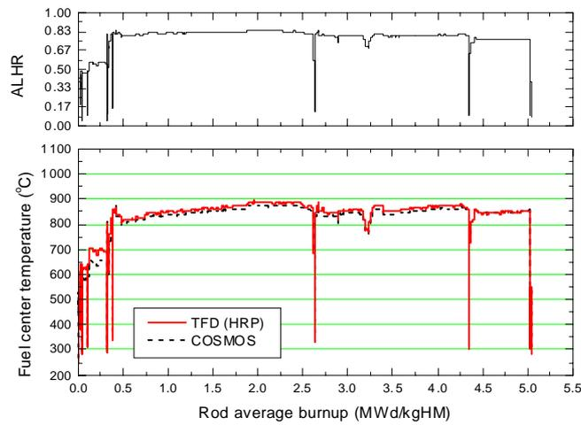
Figure 9. Comparison of COSMOS calculated centerline temperature with measured values for MOX-ATT-TF
