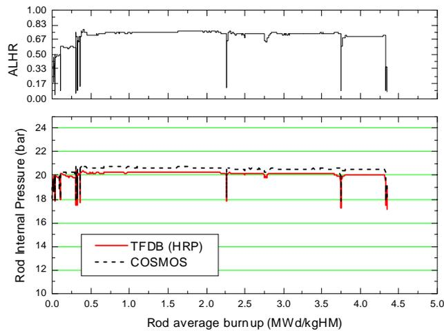
Figure 12. Comparison of COSMOS calculated RIP with measured values for MOX-ATT-ET
