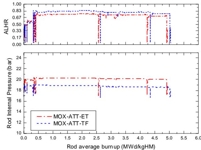
Figure 4. Variation of measured rod internal pressure.
