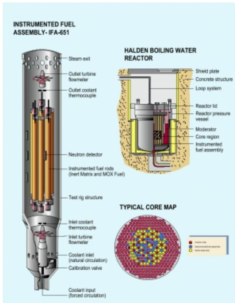
Figure 1. Schematic of IFA-651 rig and Halden Boiling Water Reactor
