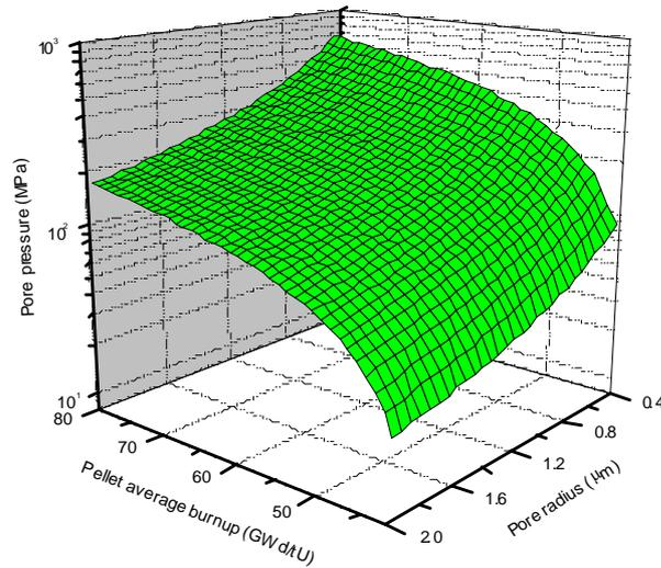
Figure 8. Calculated pore pressure in the rim as a function of pellet average burnup and pore radius.
