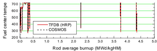
Figure 11. Comparison of COSMOS calculated centreline temperature with measured values for MOX-ATT-ET
