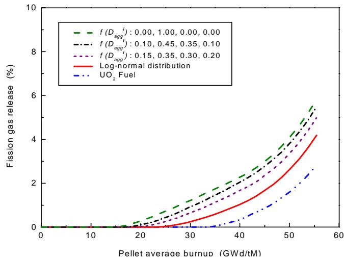
Figure 6. Effect of the size distribution of Pu-rich particles  $f(D_{agg}^i)$  on fission gas release in a MOX pellet with 4 groups of Pu-rich particles. ( $N_{agg} : 0.5 \times 10^{13}$ ,  $f_{Pu} : 0.3$ ,  $D_{agg}^i : 15, 30, 45, 60 \mu\text{m}$ )
