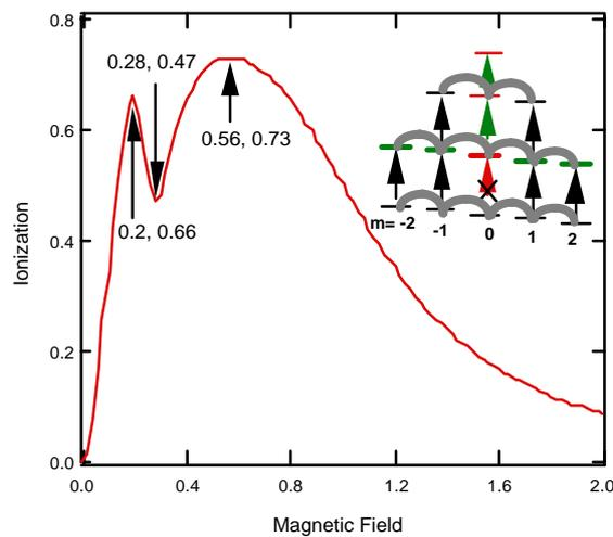
Fig. 3 Magnetic field dependence of ionization. Because of the interference between Rabi and Larmor frequency, a dip appears in this graph. Pair of Arabic numerals in graph present the magnetic field and ionization, respectively.
