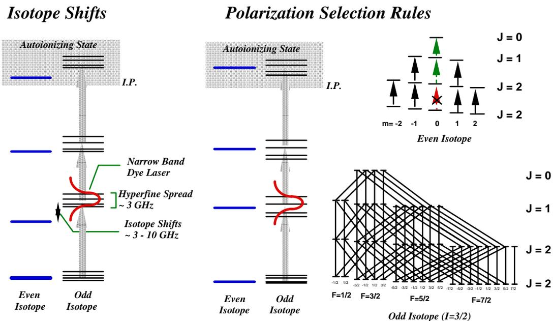
Fig.1 Three-step photo-ionization scheme based on (a) isotope shifts and (b) polarization selection rule.
