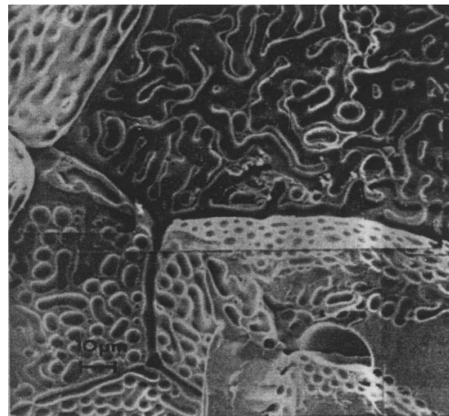
b) SEM of the fracture surface of Cr 2 O 3 -doped UO 2 , Of grain size 70 micron, irradiated to 0.28% FIMA burnup at 1460°C showing the formation of snake-like pores created by the coalescence of lenticular grain Face gas bubbles
