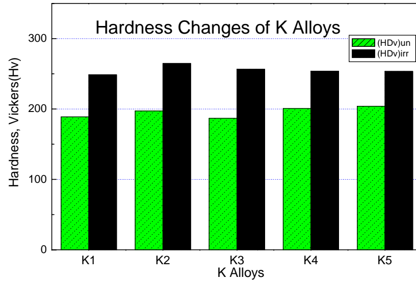
Fig. 5 Changes of Hardness of new K alloys before and after irradiation
