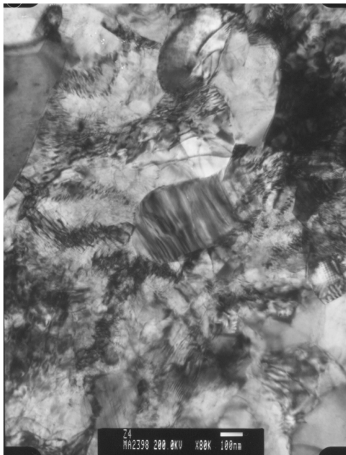
Fig. 2 TEM microstructures of the unirradiated Zircaloy-4 fuel cladding
