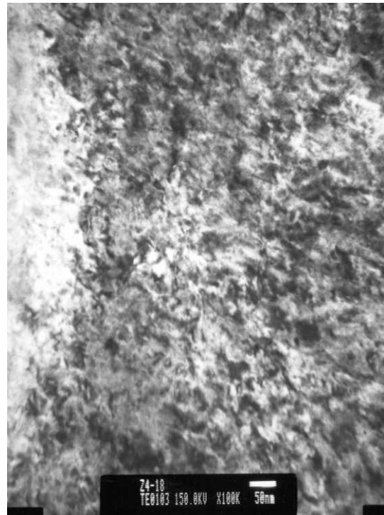
Fig. 8 Dislocation loop of a-type in the low burn-up sample (18 GWD/MTU)
