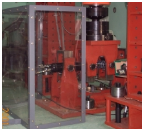
Fig. 3 Photograph of 4 points loading frame with pipe specimen.
