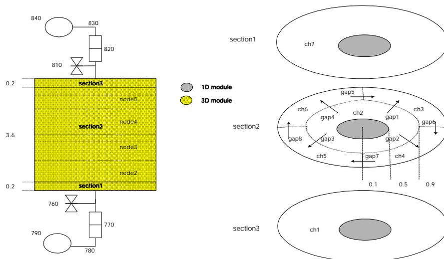
Figure 4. 3D Quenching tank nodalization
