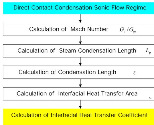
Figure 2. Calculation procedure of DCC models in sonic flow regime
