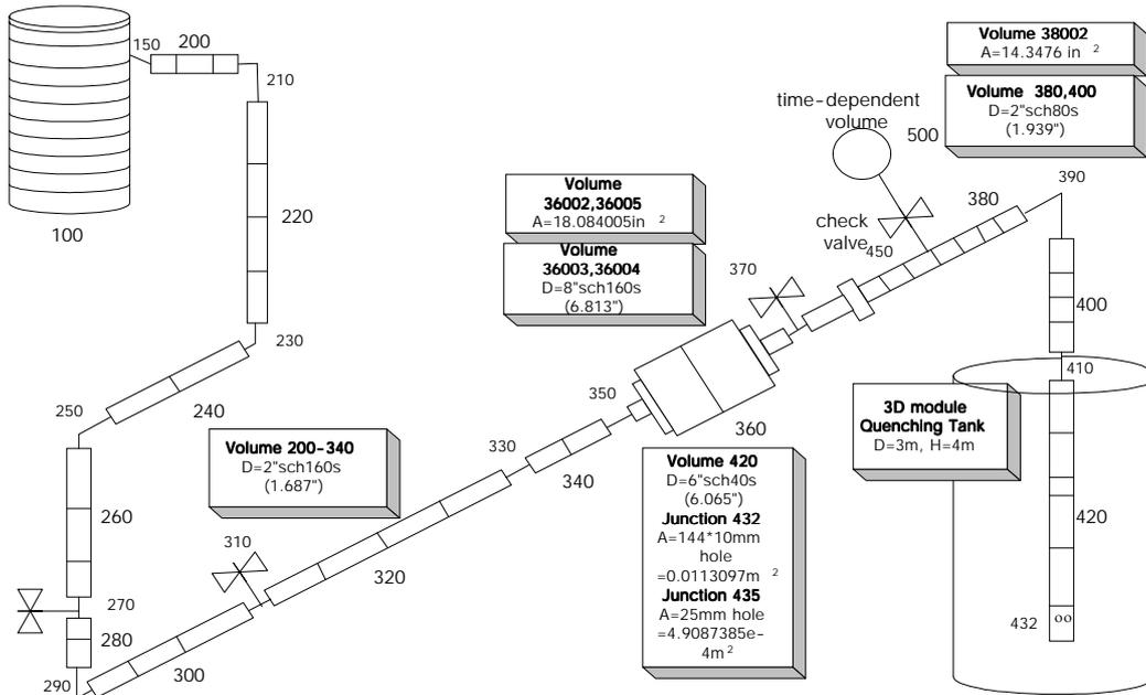
Figure 3. 1D nodalization for unit cell test facility
