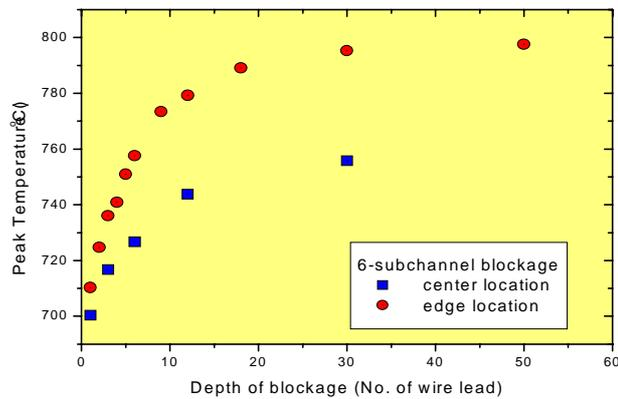
Fig.9 Peak temperatures of 6 subchannel blockages
