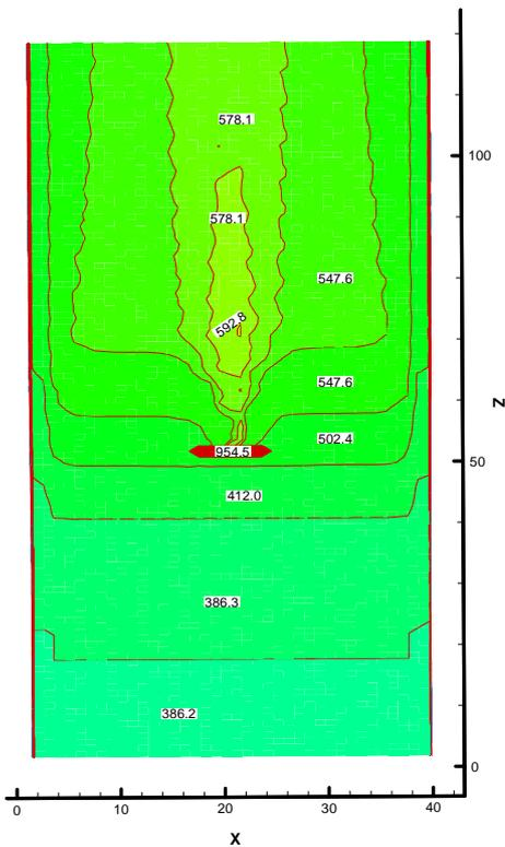
Fig. 8 Temperature contour in x-z plane for central 24 subchannel blockage
