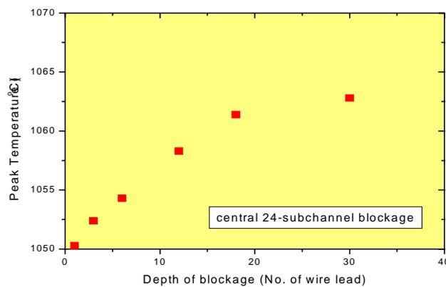
Fig.10 Peak temperatures of 24 subchannel blockages
