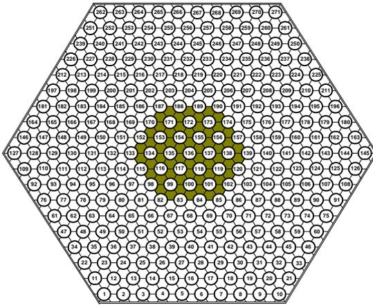
Fig.4 Central 24-subchannel blockage
