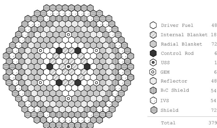
Fig. 1 Layout of KALIMER breeder core
