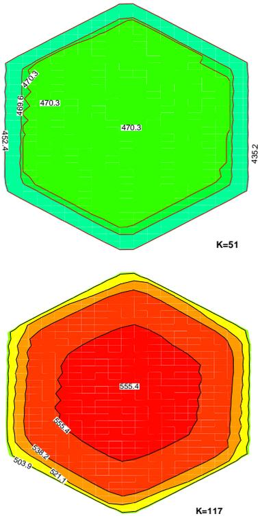
Fig.6 Temperature contour at steady state (K=51, 117)
