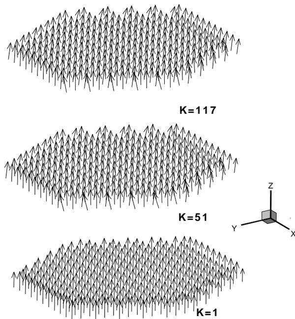
Fig. 5 Velocity vectors at inlet, mid, and outlet location of subassembly
