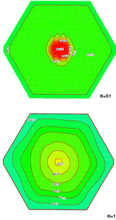
Fig.7 Temperature contour for central 24 subchannel blockage
