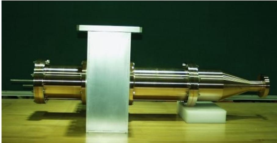
Figure 5. The fabricated Coaxial-type input RF coupler.
