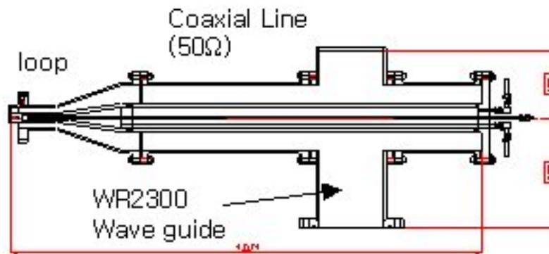
Figure 1. Drawing of the coaxial-type input coupler.
