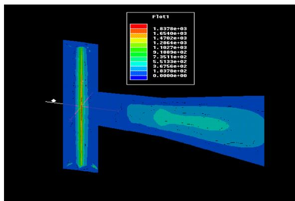
Figure 8. Electric field distribution in the RFQ and input RF coupler
