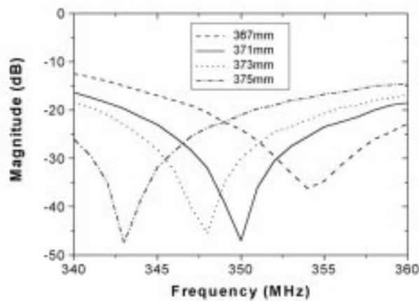
Figure 3. Return loss versus the position of short plate of the coaxial line.
