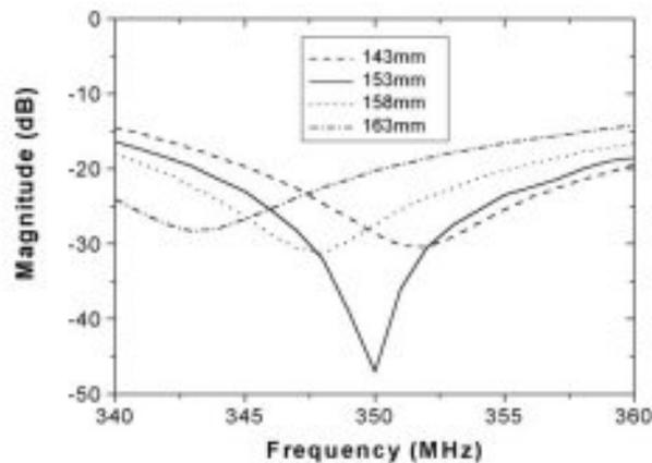
Figure 2. Return loss versus the position of short plate of the waveguide.
