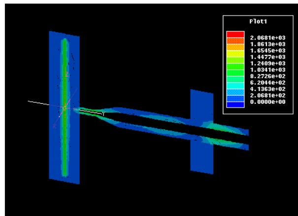
Figure 4. Electric field distribution in the matched RFQ and input coupler.
