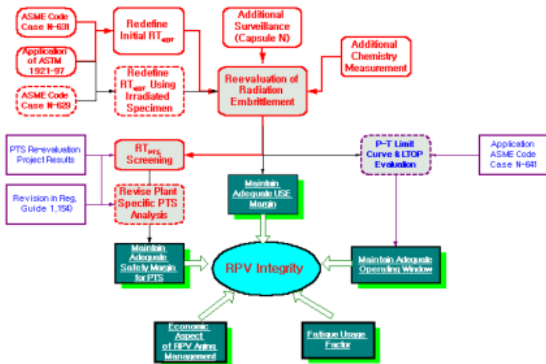
Figure 5. The Various Aspects of the RPV Integrity Assessment for Life Extension (Boxes with the dotted line are the work to be done)
