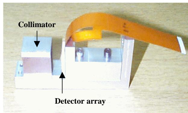
Figure 1: A photograph of 16-channel sample detector array, which consists of  $\text{CdWO}_4$  scintillators and silicon photodiodes with a p-i-n structure. The detector array sits on the aluminum mount and the x-ray beam collimator is also included.
