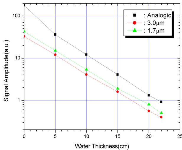
Figure 4: Signal output of the CT detector ( $\text{CdWO}_4$  + p-i-n photodiode) when irradiating x-rays for various water depths. For the comparison, the commercial Analogic CT detector was also evaluated at the same condition.
