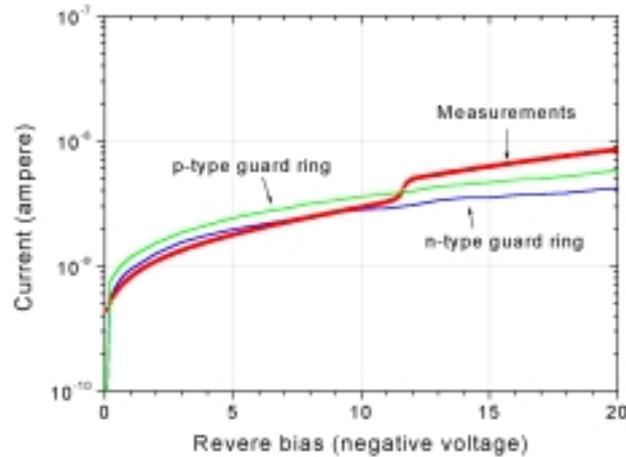
Figure 2: Dark reverse leakage current of the p-i-n photodiode with respect to the applied reverse bias voltage. In our design, an n-type guard ring was considered. The simulation results for both of the n-type and p-type guard-rings are also included for the comparison.
