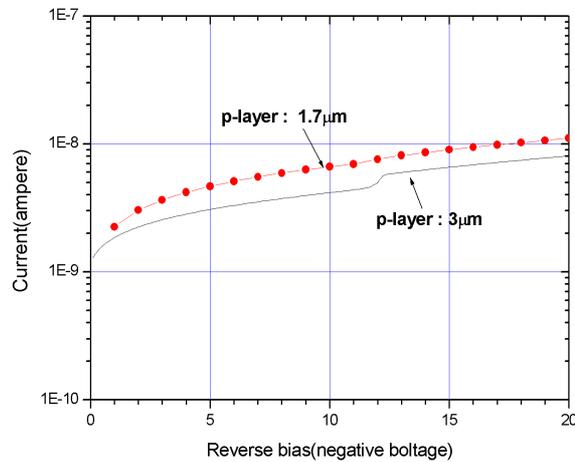
Figure 3: Dark reverse leakage current of the p-i-n photodiode as function of the applied reverse bias voltage under different p-layer thickness
