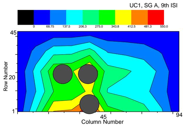
Fig. 10 Contour map of ratio of crack signals/number of tubes in SG A of plant C.(Hatched areas are SCC susceptible region)
