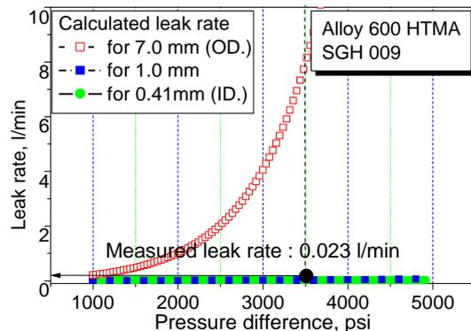
Fig. 6 Calculated and measured leak rate on the tube SGH009.
