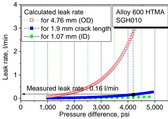
Fig. 7 Calculated and measured leak rate on the tube SGH010.
