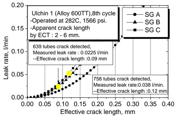
Fig. 8 Estimated effective crack length of the 8th cycle of Ulchin 1 based on the leak rate model.
