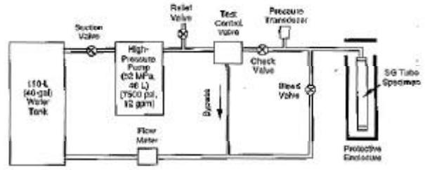
Fig. 1 Schematic of the pressure test facility.
