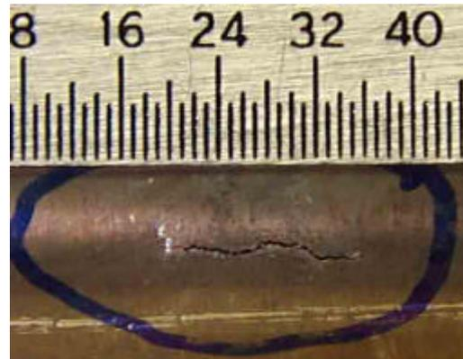
Fig. 4 Flaws on the SGH005 after the room temperature pressure/leak test.
