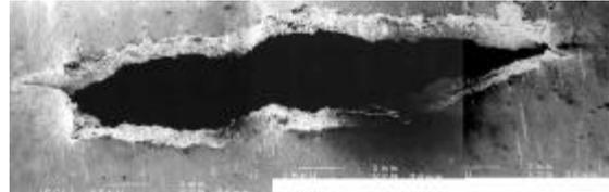
Fig. 2 Crack morphology of SGH002 after the pressure/leak test at room temperature.
