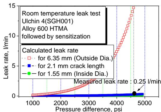
Fig. 5 Calculated and measured leak rate on the tube SGH001.
