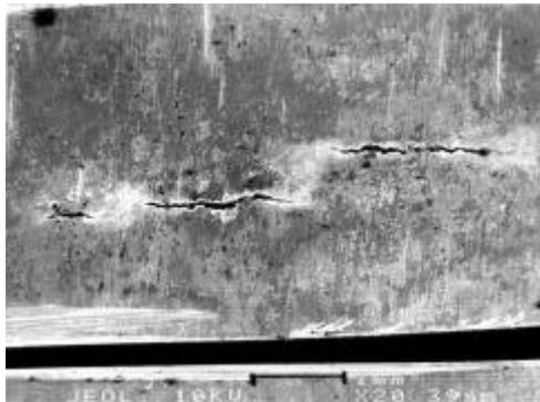
Fig. 3 Flaws on the SGH001 after the pressure/leak test at room temperature.
