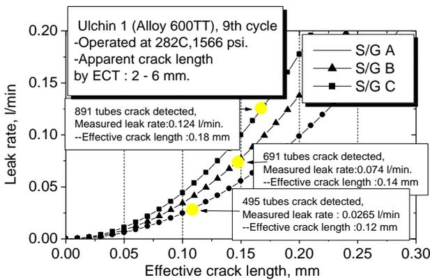
Fig. 9 Estimated effective crack length of the 9th cycle of Ulchin 1 based on the leak rate.
