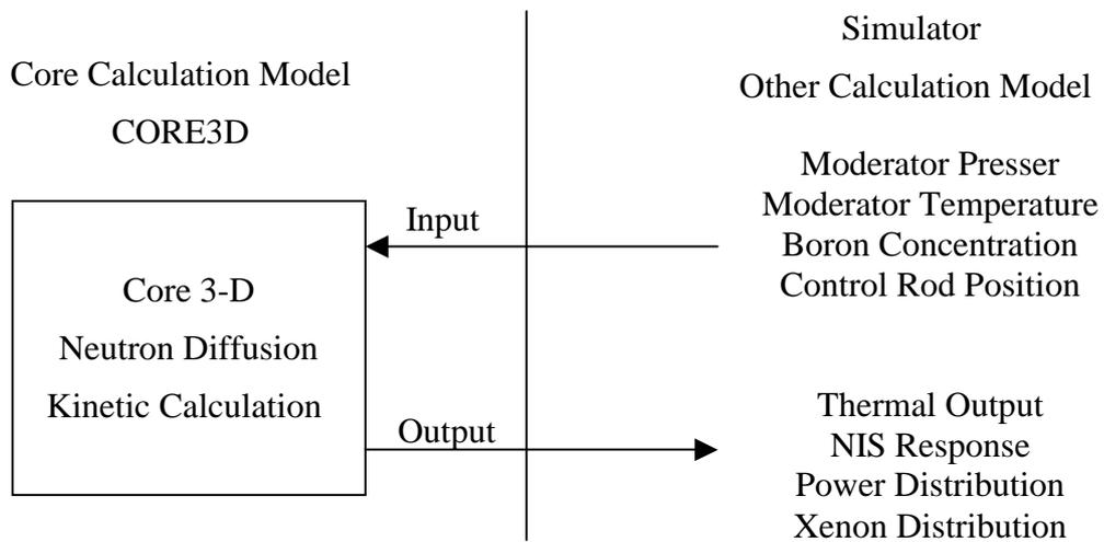
Figure 2-1 Interface between CORE3D and Other Calculation Model
