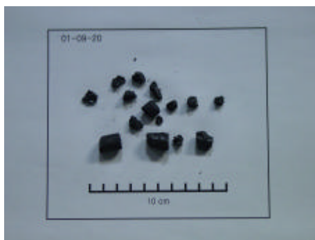
16. UO2 pellets in the debris in TROI-11
