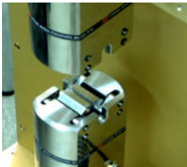
Fig. 4.7 Wedge type gripper of elongation tester
