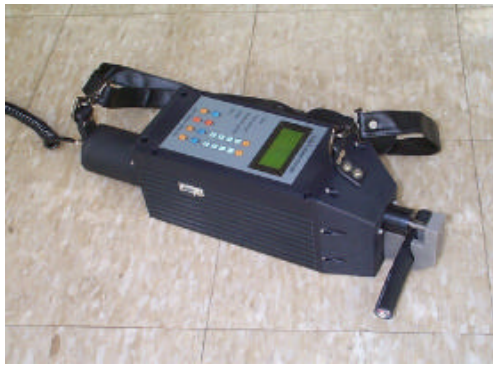
Fig.4.9 Picture of cable indenter(KEPRI made)
