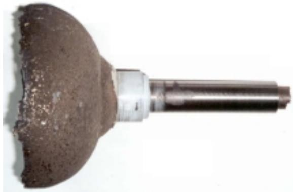
Fig. 4. Broken zirconia sleeve by thermal expansion.
