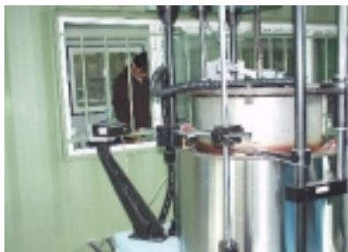
Fig. 5 Laser displacement sensor for measuring the residual displacement
