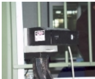
Fig. 5 Laser displacement sensor for measuring the residual displacement
