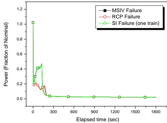
Figure 13. Core Power(Fraction of nominal)
