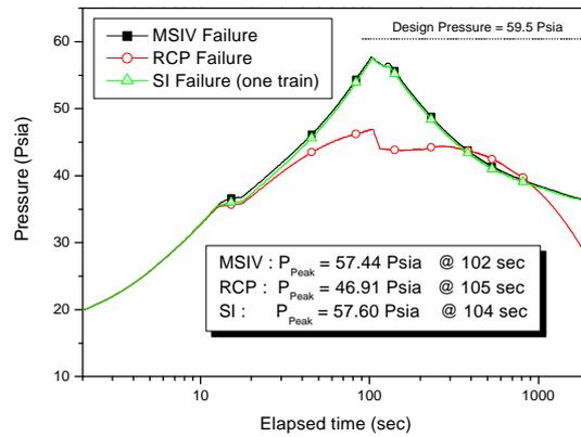
Figure 17. Single Failure (For Pressure)
