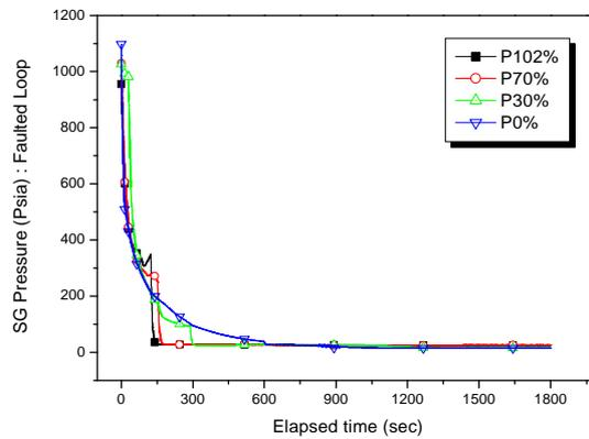
Figure 10. Steam Generator Pressure : Faulted Loop
