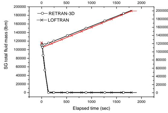
Figure 5. Steam Generator Total Fluid Mass
