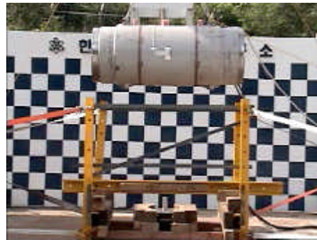
Figure 7. 1 m Horizontal Puncture Drop Test
