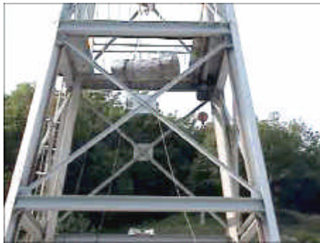
Figure 6. 9 m Horizontal Free Drop Test
