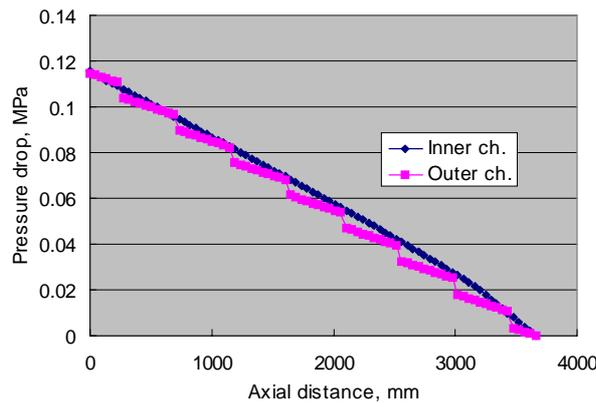
**Figure 7 Hottest cell axial pressure drop profiles for the WASB-A\_A**
