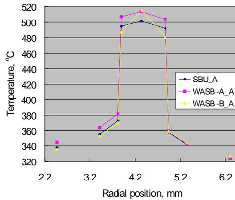
**Figure 12 Radial temperature profiles at the hottest axial positions in the hottest annular seed pins**
