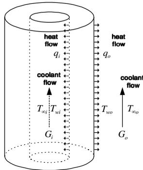
Figure 1 Annular fuel pin
