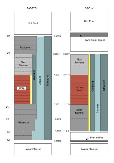
Note: K1 ~ k6 are Orifice coefficients defined at Block 64, Loc48 -63
