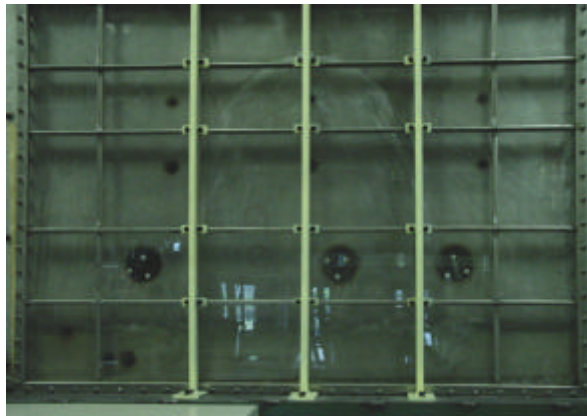
Figure 4. Experimental photo of water film width (Water mass flow rate = 1.0 kg/sec)
