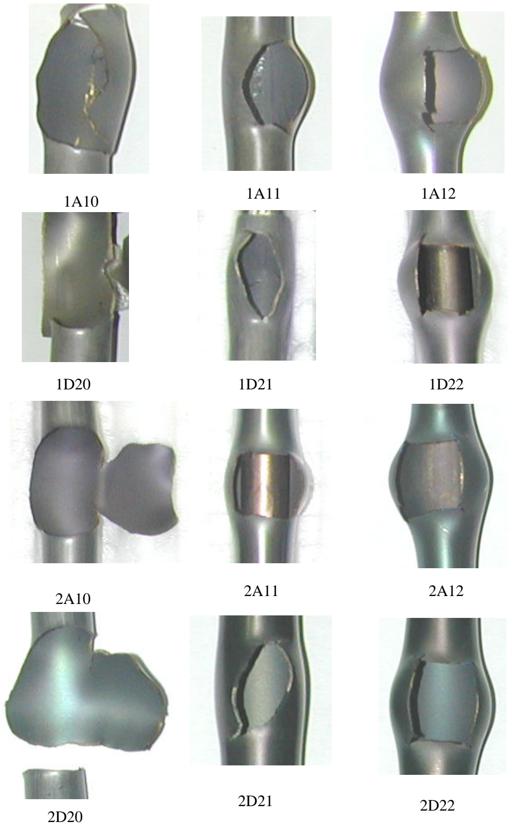
Fig. 3. Burst Fractographs of both K1 and K2 claddings: A10, A11, A12, D20, D21 and D22 at 400°C
