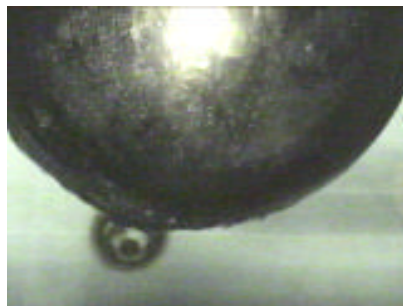
Figure 9 Visualization of Nucleate Boiling
