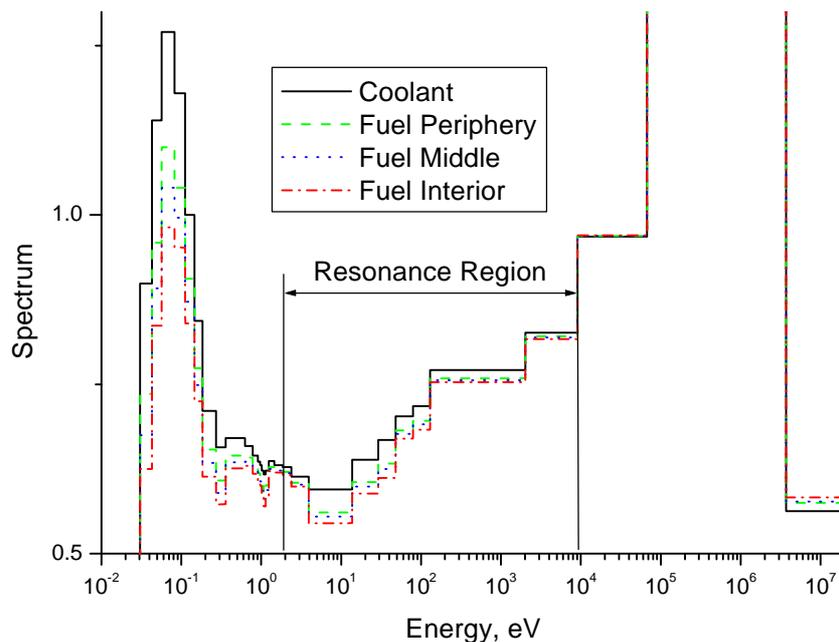
Figure 2. Typical spectrum in the moderator and fuel regions
