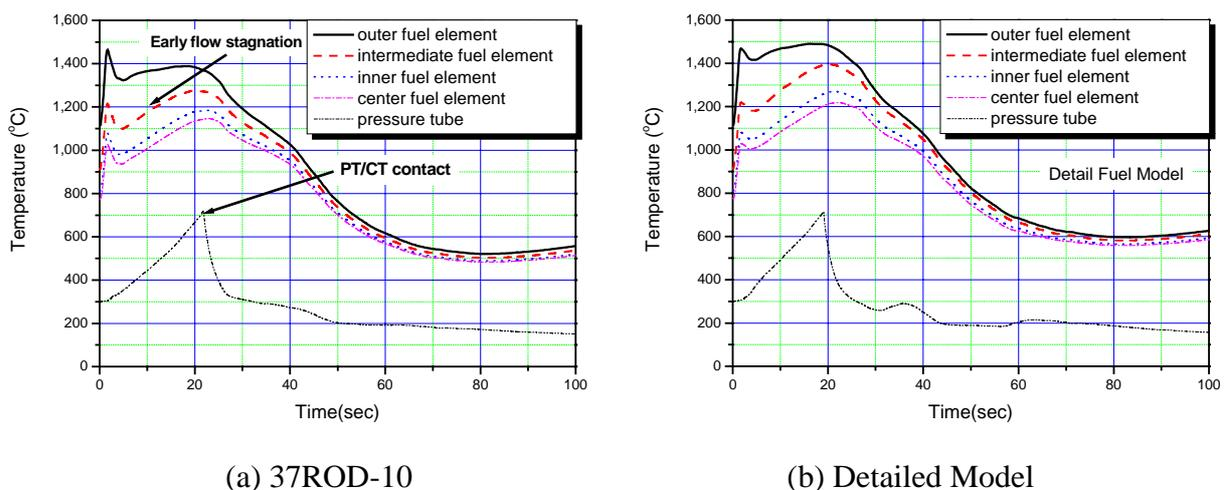
Figure 4 Fuel and Channel Temperatures in the Critical Pass for a 35% RIH Break with Loss of ECC Injection (Bundle 6 of 7.3 MW Channel)
