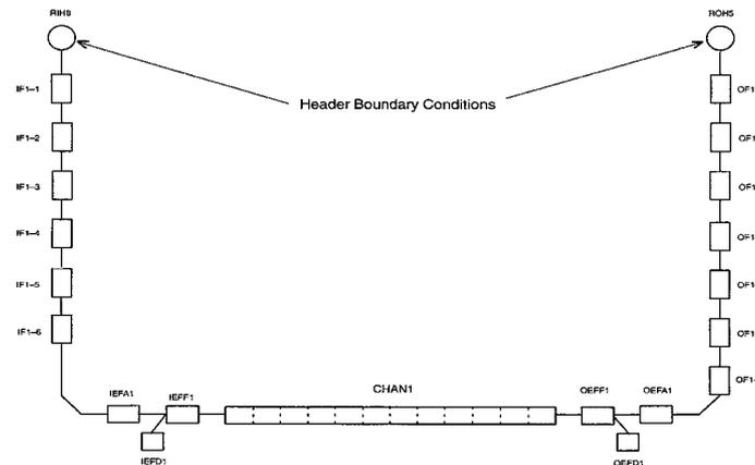
Figure 2 Nodalization of CATHENA Slave Channel Model
