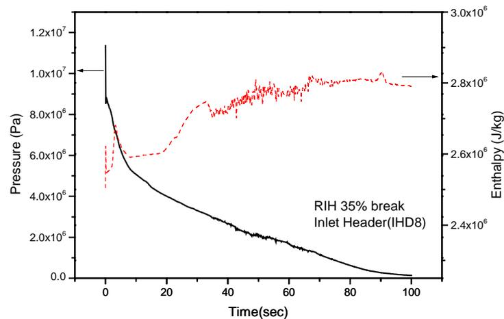
Figure 1 Header BC.s from Circuit Analysis (Critical Pass: RIH 35% break)
