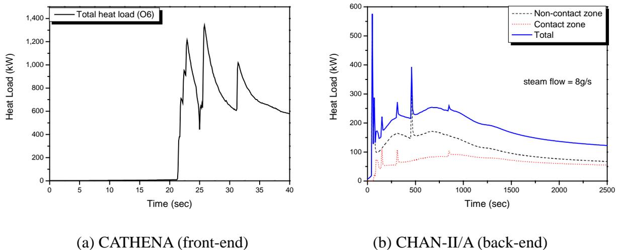
Figure 9 Heat Load from Calandria Tube to Moderator: 35% RIH Break with Loss of ECC Injection (Critical Pass of 7.3 MW Channel)
