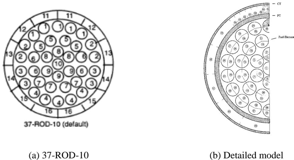
Figure 3 Fuel Pin Grouping for Channel O6
