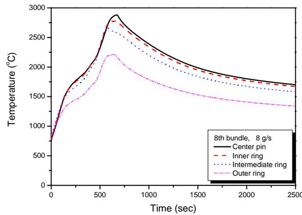
Figure 7 Ring Average Temperatures for a 35% RIH Break with Loss of ECC Injection (Critical Pass of 7.3 MW Channel)
