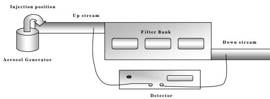
Fig. 1. Schematic diagram of in-place leak test for HEPA filter bank.
