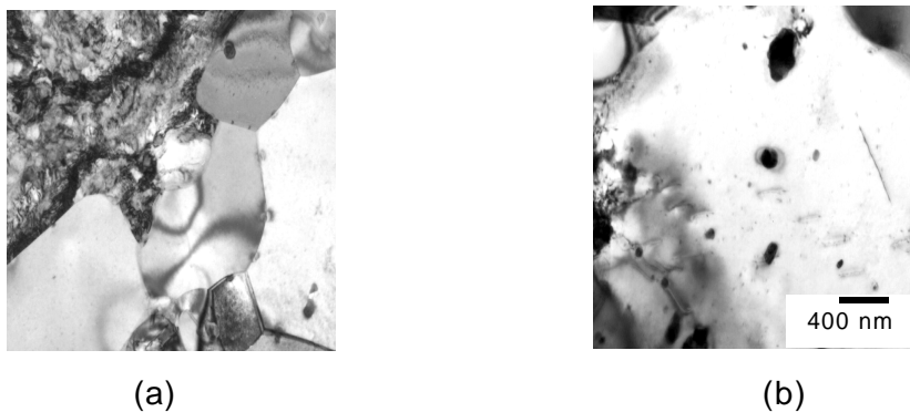
Fig. 6 TEM microstructures of Zr-0.2Nb - 1.0Sn - FeCrCu claddings with final annealing temperature; (a) 470°C, (b) 520°C
