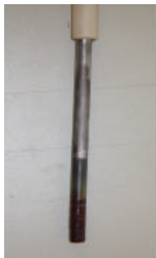
Fig. 3. Oxide of layer of platinum anode electrode.
