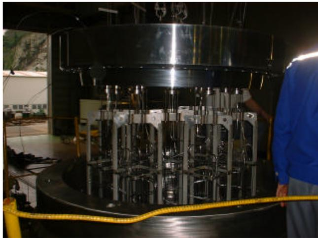
Figure 2 Test equipment(test lid, leadthroughs, dummy heaters and thermocouples)
