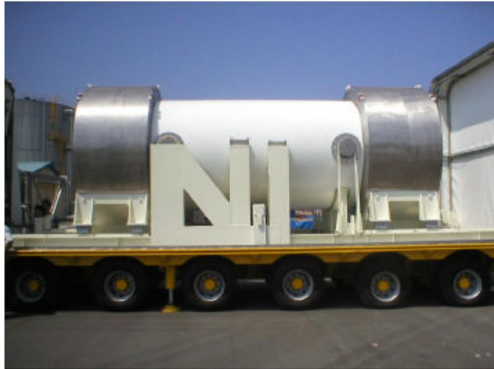
a. The cask mounted on the tie-down of the transport trailer with impact limiters
