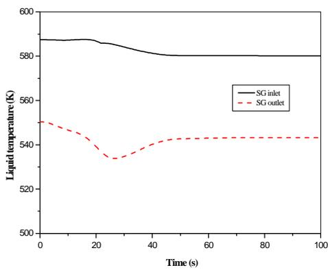
Fig. 8 Primary coolant temperature for the increased steam flow event
