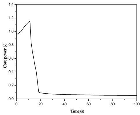
Fig. 7 Normalized core power for the increased steam flow event
