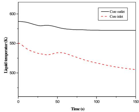
Fig. 15 Primary coolant temperature for the steam line break accident
