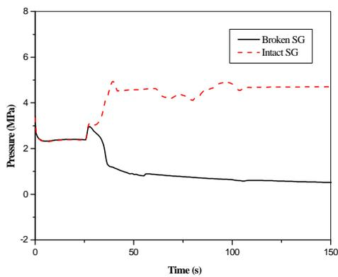
Fig. 14 Secondary system pressure for the steam line break accident
