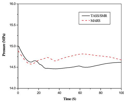
Fig. 6 Pressurizer pressure with TASS/SMR and MARS codes
