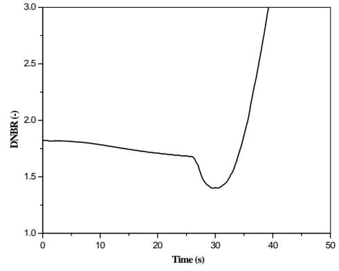
Fig. 17 DNBR for the steam line break accident
