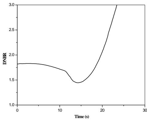
Fig. 12 DNBR for the increased steam flow event
