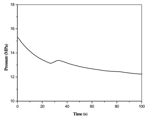
Fig. 13 Primary system pressure for the steam line break accident
