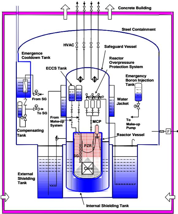
Fig. 1 Safety systems of the SMART
