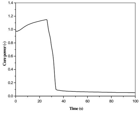
Fig. 16 Normalized core power for the steam line break accident
