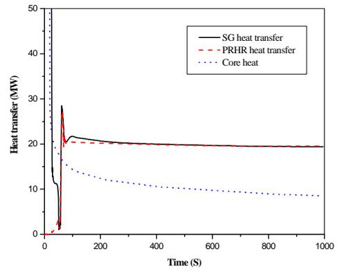
Fig. 11 Heat rate removed in RHRs for the increased steam flow event
