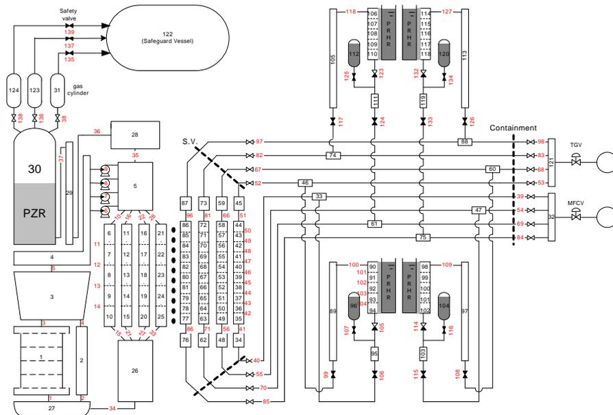
Fig. 3 TASS/SMR nodalization for the SMART
