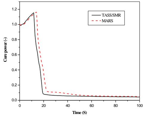
Fig. 5 Normalized core power with TASS/SMR and MARS codes
