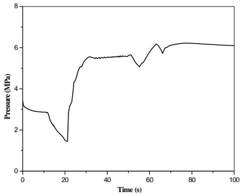
Fig. 10 Secondary pressure for the increased steam flow event
