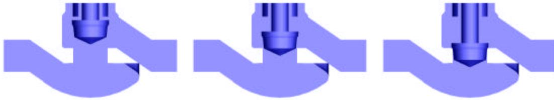
(a) open rate = 100%      (b) open rate = 50%      (c) open rate = 0%
